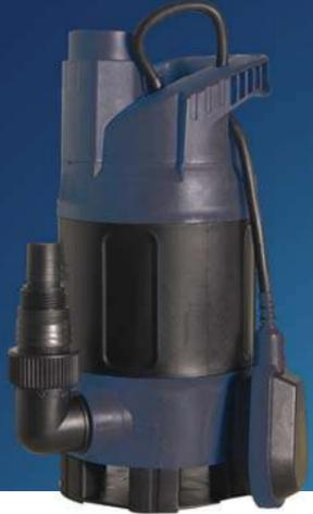
Shaft sealing between the pump and motor is accomplished by two mechanical seals and a lip seal in all the pumps in our wastewater pump product range. The pumps should be completely immersed in the fluid and use must be limited to fluids below 40°C, since the cooling of motor is done by the immersed liquid.
